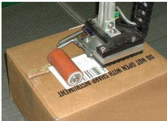
Model 250 applying a shipping label
