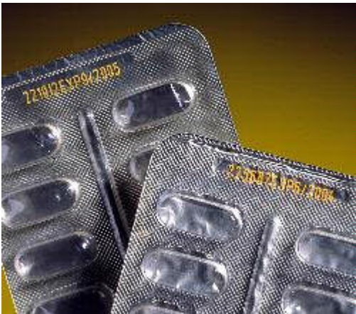
Expiration and lot codes printed with laser coder
