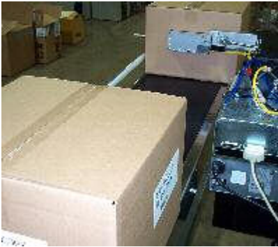
Labeling Front and Side Panel of a Case
