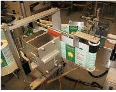
Overprinter mounted to Label Applicator
